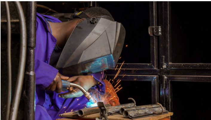
Artisan (welder) welding metal
